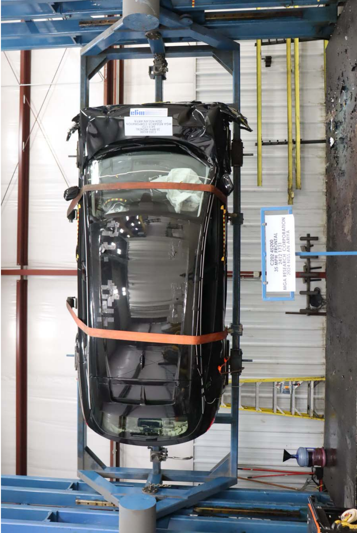
Photo No. 63. Rollover 90 Degrees
