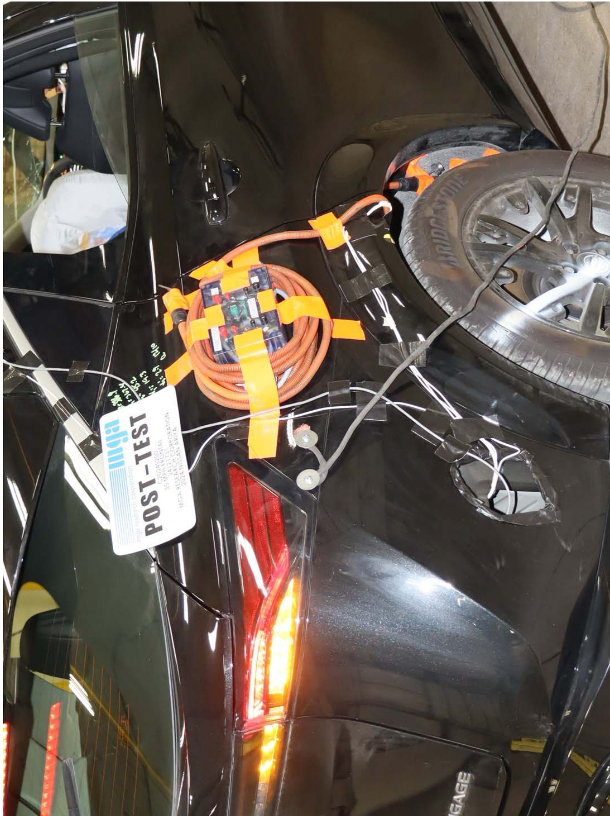
Photo No. 76. Post-Test View of Installed Isolation Interface Port
